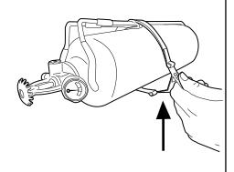
3. Place clasp around device and clip into place to secure.
