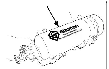
Visual check to see if there is any external damage to the device. If there are signs of corrosion the device must be removed and replaced with a new device.
