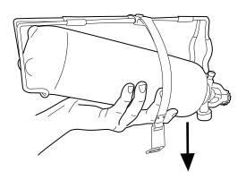
2. Release device from fixing bracket. Dispose of device. We would recommend recycling with other metal items.
