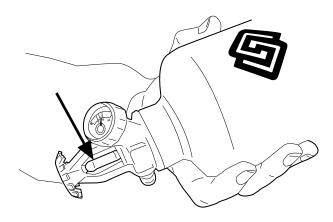
Visual check to see if the glass vial is intact. Should the device have been activated the vial will be missing, and should be replaced with a new device.
