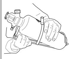
1. Remove device from new bracket as it will not be required. See above for details to remove clasp.
