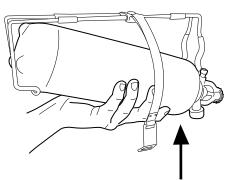
2. Offer device to bracket inside hood of bin and click into place. NOTE: The metal plate in front of the device is there to deflect the powder down into the bin.
